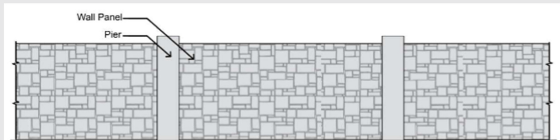
Figure 2. Elevation of Typical Noise Barrier/Sound Wall
